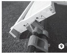
A wood clamp is handy to get your wires guitar-string tight. Place the clamp on the side bar adjacent to but not covering the eyelets. You want the wire to be able to move through the eyelets when tightening. Tighten the clamp until you can just start to see your frame bow in at the sides – enough to slacken the wire but not so tight that you crack your frame (Fig. 8). Without removing the clamp, re-tighten the wire around the bottom tack nail as tight as you can wrap it (Fig. 9).
